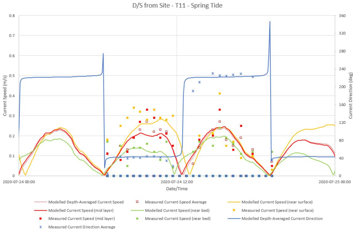
**Figure 3.6: Comparison of measured and modelled current speed and direction at ADCP transect T11 downstream of the site during Spring Tide**
