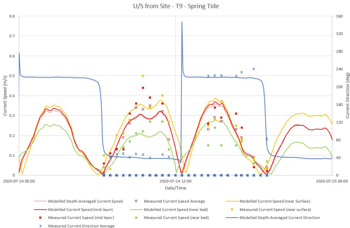
**Figure 3.4: Comparison of measured and modelled current speed and direction at ADCP transect T9 upstream of the site during Spring Tide**
