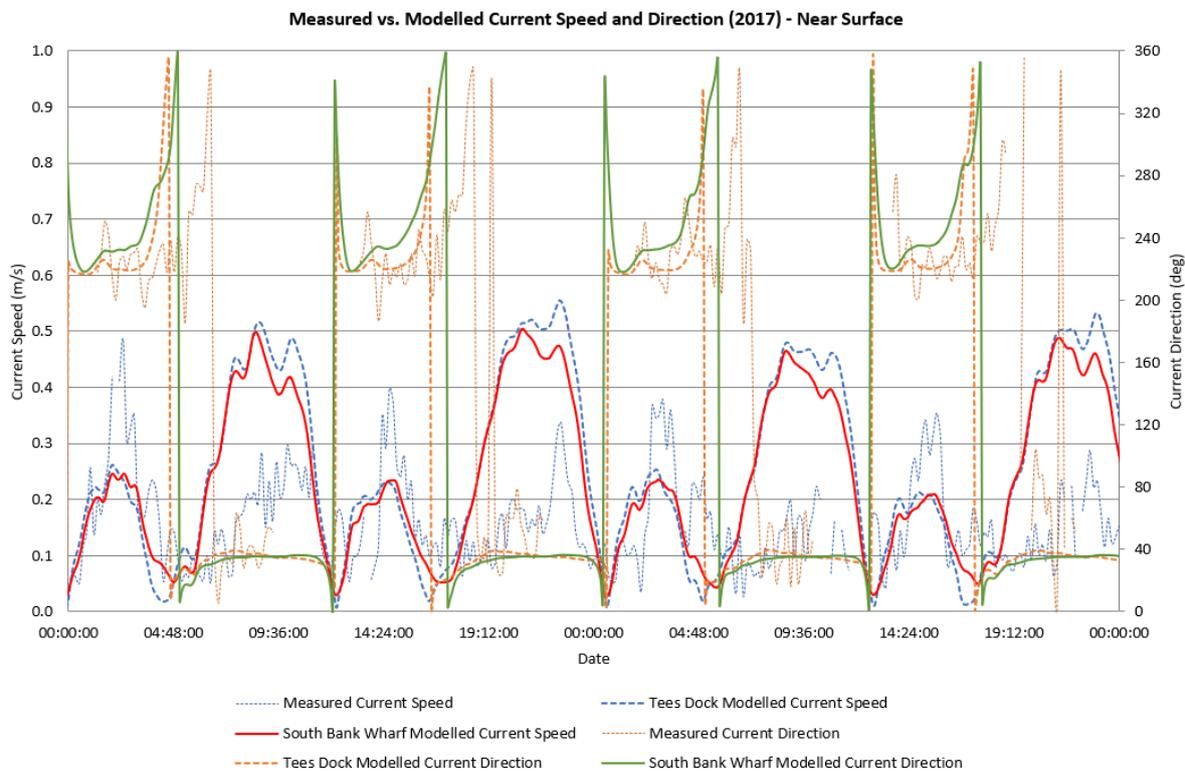
**Figure 2.18: Comparison of Measured and Modelled Current Speed and Direction near water surface**
