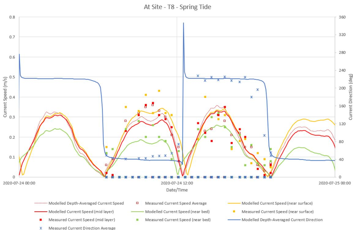
**Figure 3.5: Comparison of measured and modelled current speed and direction at ADCP transect T8 at the site during Spring Tide**
