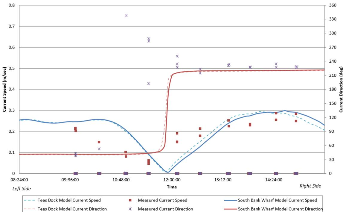
**Figure 2.13: Comparison of Measured and Modelled Current Speed and Direction at Transect 8 on 27th April 2005**
