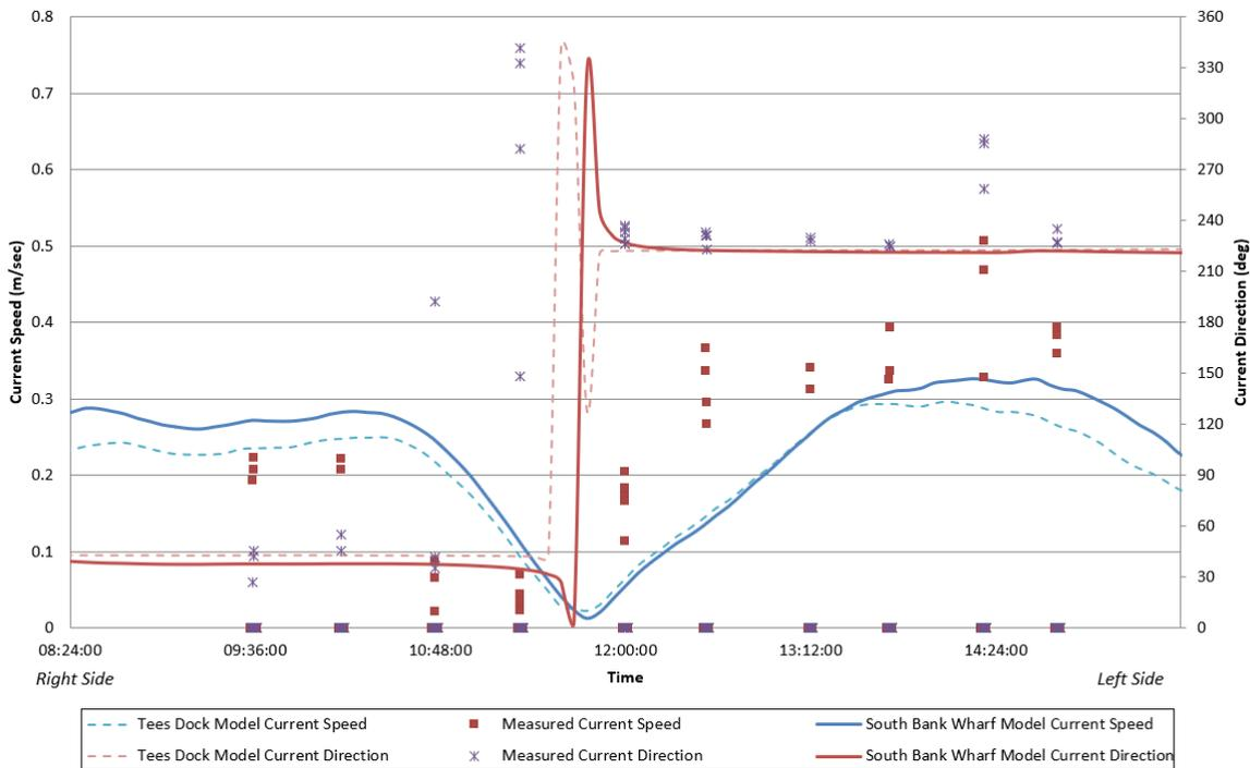
**Figure 2.12: Comparison of Measured and Modelled Current Speed and Direction at Transect 9 on 27th April 2005**
