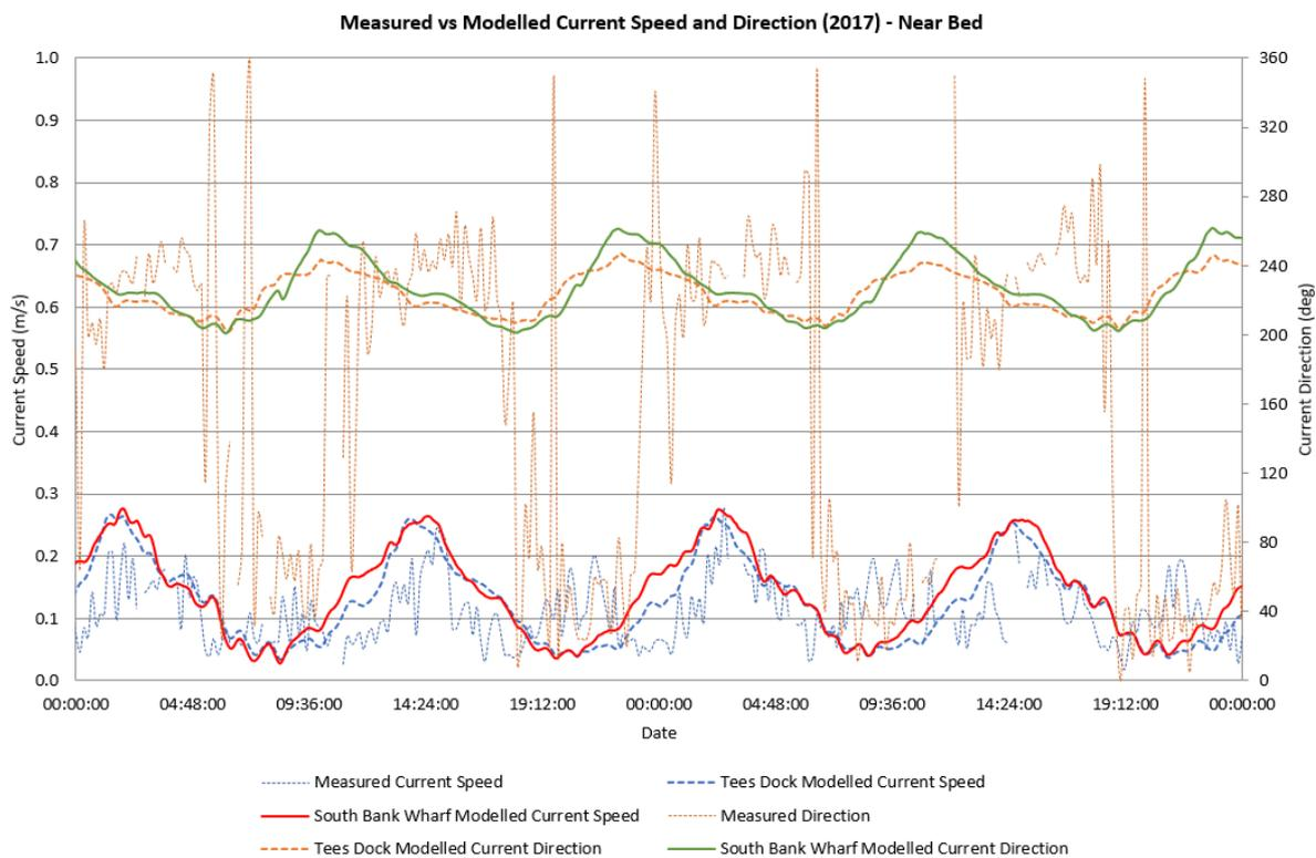
Figure 2.16: Comparison of Measured and Modelled Current Speed and Direction near bed
