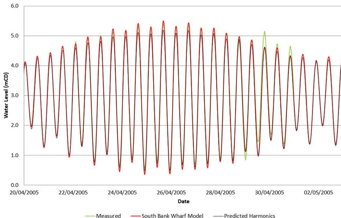
**Figure 2.11: Comparison of Measured, Modelled and Predicted Tidal Elevation at Tees Dock Tide Gauge between 22<sup>nd</sup> to 30<sup>th</sup> April 2005**
