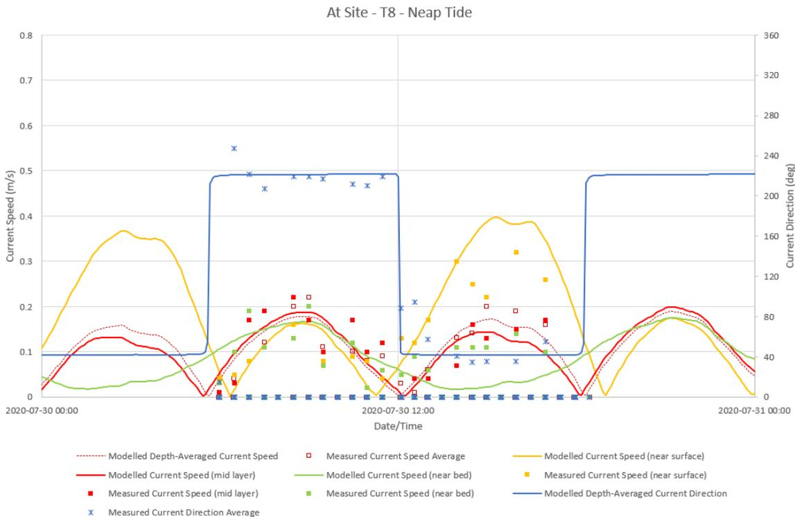
**Figure 3.8: Comparison of measured and modelled current speed and direction at ADCP transect T8 at the site during Neap Tide**
