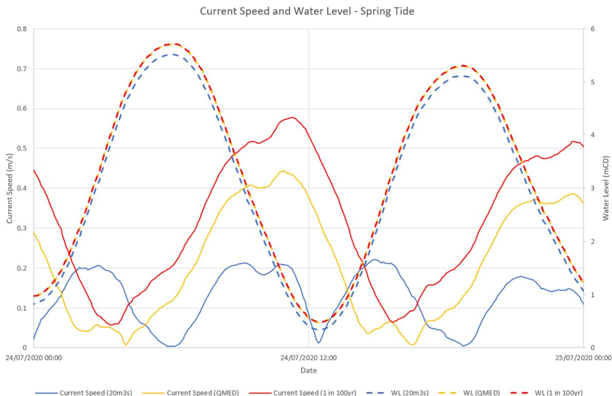
**Figure 4.3: Current Speed and Water Level during Spring Tide at Site**
