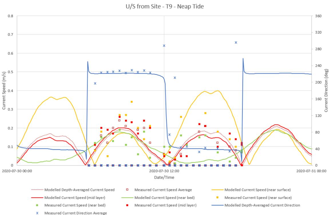
**Figure 3.7: Comparison of measured and modelled current speed and direction at ADCP transect T9 upstream of the site during Neap Tide**
