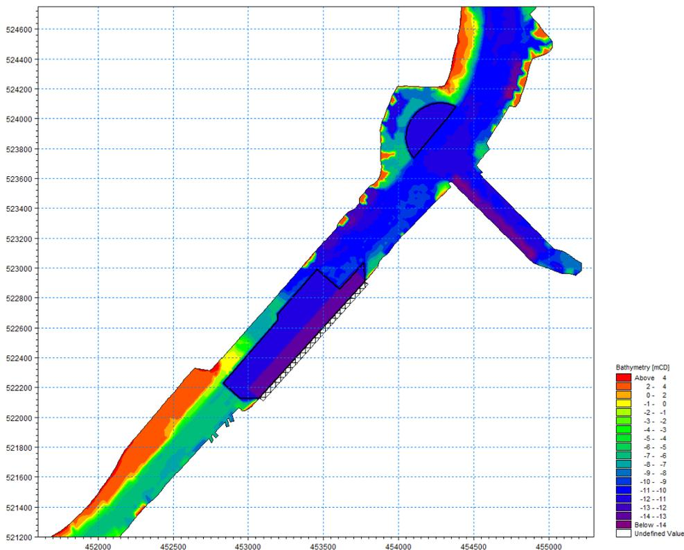
Figure 4.2: Model Scheme Bathymetry
